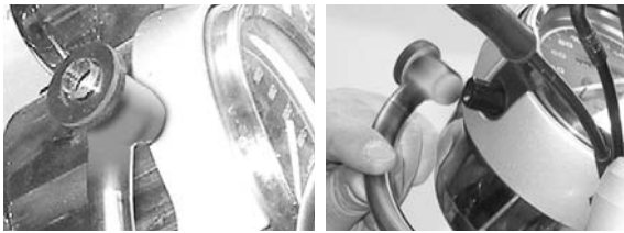
Rubber washer should not overhang edge of mount.
